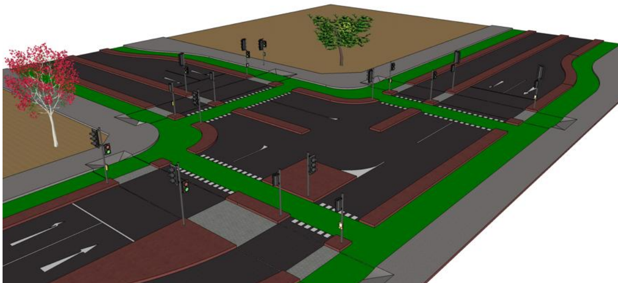
3-D model of a possible UK traffic-controlled junction, with separate cycle tracks. Signal arrangements keep the movements of motor vehicles and cyclists separate. Courtesy of LCC Croydon Cycling Campaign
